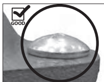
OVAL NECK OF BOLT SEATED PROPERLY
