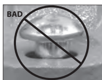
OVAL NECK OF BOLT NOT SEATED PROPERLY
