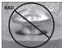
OVAL NECK OF BOLT NOT SEATED PROPERLY
