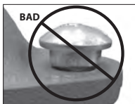
OVAL NECK OF BOLT NOT SEATED PROPERLY
