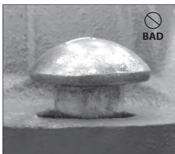
BAD BOLT ENGAGEMENT (OVAL NECK IS NOT SEATED PROPERLY IN THE BOLT HOLE)
