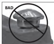
OVAL NECK OF BOLT NOT SEATED PROPERLY
