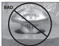
OVAL NECK OF BOLT NOT SEATED PROPERLY
