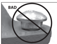
OVAL NECK OF BOLT NOT SEATED PROPERLY
