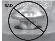
OVAL NECK OF BOLT NOT SEATED PROPERLY
