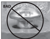
OVAL NECK OF BOLT NOT SEATED PROPERLY
