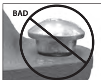
OVAL NECK OF BOLT NOT SEATED PROPERLY
