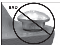
OVAL NECK OF BOLT NOT SEATED PROPERLY
