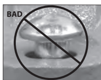
OVAL NECK OF BOLT NOT SEATED PROPERLY
