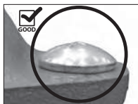
OVAL NECK OF BOLT SEATED PROPERLY
