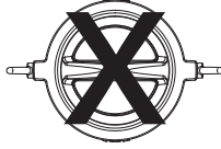
Incorrect Orientation for Horizontal Installation
