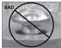
OVAL NECK OF BOLT NOT SEATED PROPERLY
