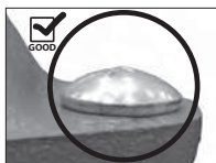
OVAL NECK OF BOLT SEATED PROPERLY
