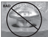
OVAL NECK OF BOLT NOT SEATED PROPERLY
