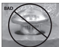
OVAL NECK OF BOLT NOT SEATED PROPERLY
