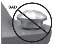
OVAL NECK OF BOLT NOT SEATED PROPERLY
