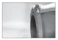
**3. ADD ADDITIONAL SEGMENTS:** Add each segment by inserting the draw bolts (provided) into the flange adapter with the nuts (provided) loosely and uniformly tightened. This will permit the flange adapter to be rotated for bolt hole alignment in later steps.
