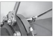
**11. TORQUE ASSEMBLY BOLTS:** Tighten all assembly bolts evenly until the required torque value is achieved. Refer to the "Style 741 Assembly Bolt Torque Requirements" table below for the torque requirement.
