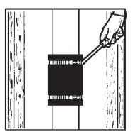
Tighten clamps to 60 inch-lbs. of torque.
