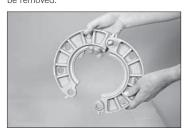
2. INSERT MATING BOLT: Insert a standard, full-shank diameter assembly bolt through a mating hole to act as a hinge, as shown above.
