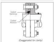
**4. INSTALL GASKET:** Install the gasket onto the pipe end. Make sure the gasket is positioned properly, as shown above. **NOTE:** The lettering on the outside of the gasket must face the gasket seating area of the Style 441 Vic-Flange Adapter.
