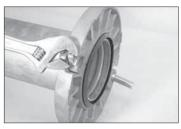
**5a.** Closure lugs are provided to ease installation. Clamp both lugs with a wrench or pliers, and pull the two segments together until the bolt holes align.
