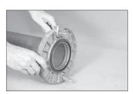
**5b.** When the bolt holes are aligned, insert a standard, full-shank diameter assembly bolt through the other mating hole of the Vic-Flange Adapter.
