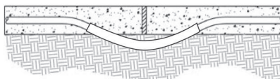
FOR CUT EXPANSION JOINTS, DIP THE TUBING BELOW THE SLAB TO A SAFE DISTANCE AT THE CUT LINES
