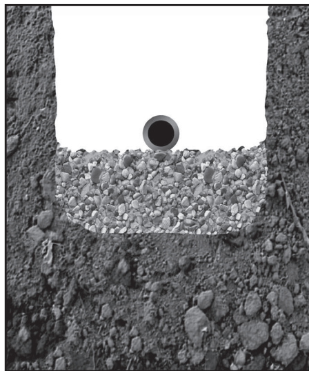
Trench in poor soil
