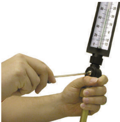
Loosen single screw (A).
