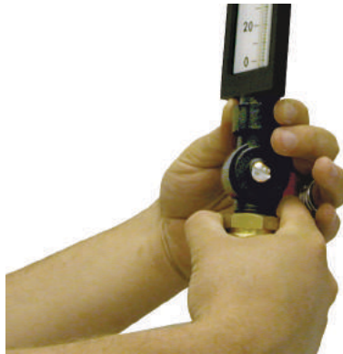
Rotate locking nut by hand.
