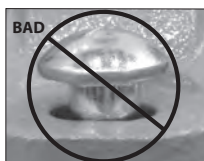
OVAL NECK OF BOLT NOT SEATED PROPERLY
