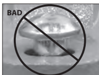
OVAL NECK OF BOLT NOT SEATED PROPERLY
