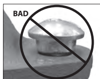
OVAL NECK OF BOLT NOT SEATED PROPERLY
