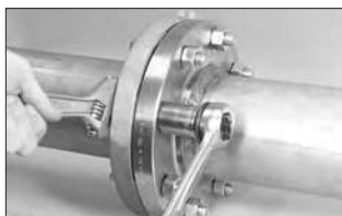
4-Bolt Tightening Pattern
