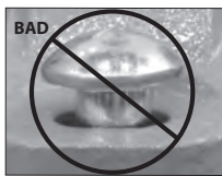
OVAL NECK OF BOLT NOT SEATED PROPERLY
