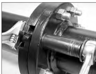
4-Bolt Tightening Pattern
