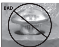
OVAL NECK OF BOLT NOT SEATED PROPERLY
