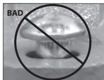
OVAL NECK OF BOLT NOT SEATED PROPERLY
