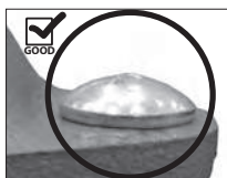
OVAL NECK OF BOLT SEATED PROPERLY
