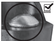
OVAL NECK OF BOLT SEATED PROPERLY
