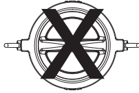
Incorrect Orientation for Horizontal Installation
