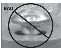
OVAL NECK OF BOLT NOT SEATED PROPERLY
