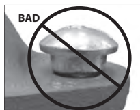
OVAL NECK OF BOLT NOT SEATED PROPERLY
