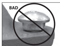
OVAL NECK OF BOLT NOT SEATED PROPERLY
