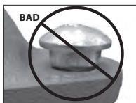
OVAL NECK OF BOLT NOT SEATED PROPERLY
