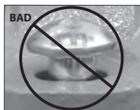
OVAL NECK OF BOLT NOT SEATED PROPERLY
