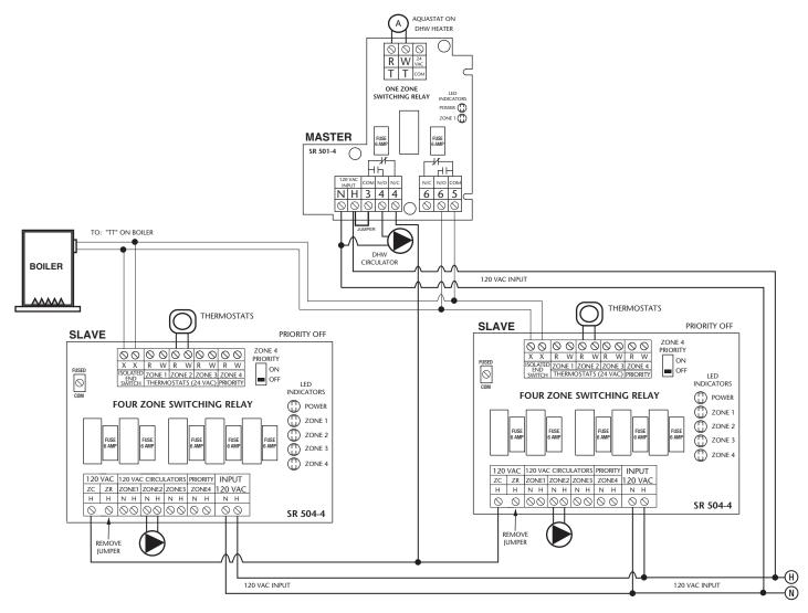
Replacement Switching Relay fuses part number: SR6A-001RP (Manufacture: Littlefuse, Part Number: 229006) Optional power stealing thermostat resistor part number: SRTR-001RP (Value: 1000 Ohms, 1/2 watt or higher)
