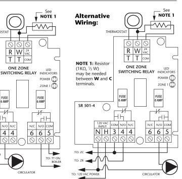
**NOTE 2:** When using Alternative Wiring diagram, the boiler operating control's ZC terminal will see the load of the circulator(s).
