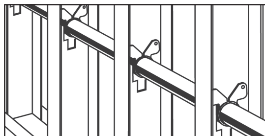
Suspension clip fasteners used to protect tubing from abrasion when passing through steel studs
