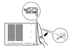
16) Take out the air filter and secure it with 2 Type A screws through the front grille.
