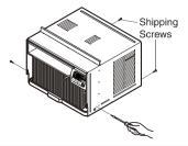
2) Slide the unit from the cabinet by gripping the base pan handle and pulling forward while bracing the cabinet.
