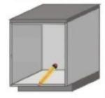
Mark drain hole position on cabinet, drill 3/8" hole for drain cone. Cut tip off drain cone.
