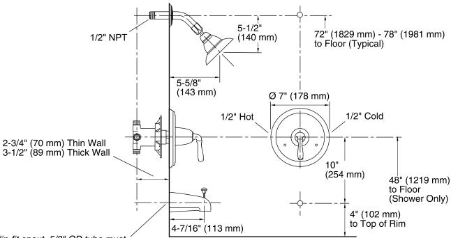
For slip-fit spout, 5/8" OD tube must extend 3-1/4" (83 mm) max beyond the finished wall.
