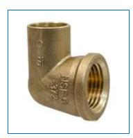
**Specifications UPC** Code 039923338136 **All Type of Item** Fitting **All Special Application** Lead-Free\* **Description** 707-3R-LF 1X1/2 CXF 90 ELB CAST **Fitting Bend Angle** 90 Deg (1/4 Bend) Elbow **Type Connection Type** C x F (NPT) Weight 0.322 lb Size 1 x 1/2 Material Lead-Free Bronze
