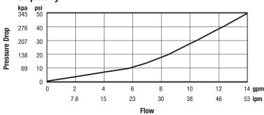
Flow curves are for reference. Actual flows may vary depending on system temperatures and/or pressures. \*\*Flow curve with integral inlet filters and check valves
