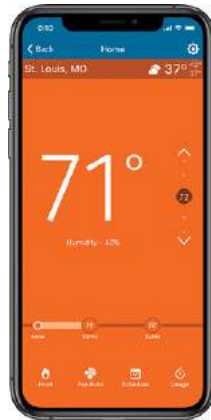
The app changes color to let you know at a glance whether the system is heating or cooling.
