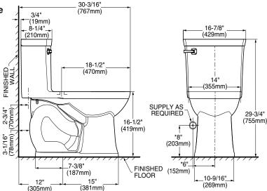
THIS TOILET IS DESIGNED TO ROUGH-IN AT A MINIMUM DIMENSION OF 305MM (12") FROM FINISHED WALL TO C/L OF OUTLET. SUPPLY NOT INCLUDED WITH FIXTURE AND MUST BE ORDERED SEPARATELY.
