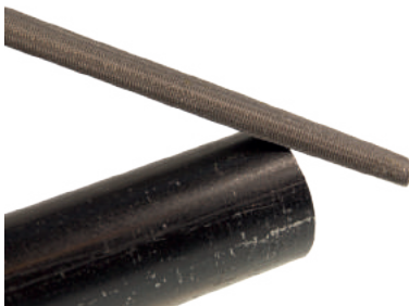
FIGURE 7: DEBURRING THE PIPE
