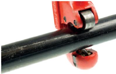
FIGURE 6: CUTTING THE PIPE
