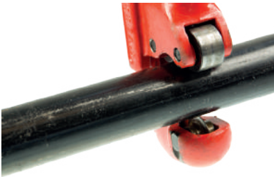
FIGURE 6: CUTTING THE PIPE
