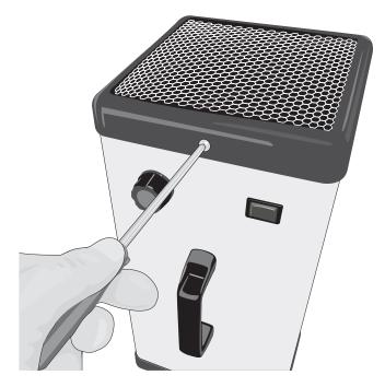
Gently remove the Plastic End Cap, screen and carbon filter. Place used carbon filter in a plastic bag and dispose of.
