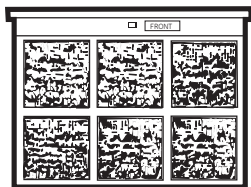
Dirty filter— Needs cleaning
