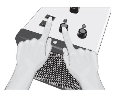
When done, press the Power Switch to the OFF position and the fan and UV bulbs will turn off.
