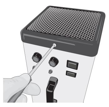
Remove five countersunk Phillips head machine screws, located on each side of upper cabinet and one placed between handle and control panel. Lift upper cabinet cover clear of the machine.
