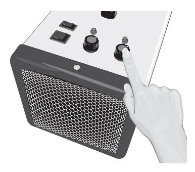
**OZONE**: (Can only be used when Hydroxyl Timer is set also, and room must be empty of people, pets and plants). Set the desired ozone time using OZONE TIMER Knob, then press the OZONE TIMER knob to the desired time; the CAUTION OZONE ON indicator will light.
